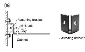
Fastening the cabinet at the top with brackets (side view)
