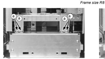
(a) M6x16 combi screws Tightening torque: 5 Nm (3.7 lbf ft)
