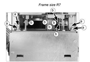
(a) M6 combi screw Tightening torque: 5 Nm (3.7 lbf ft)
