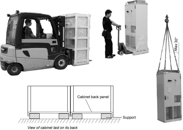
It is allowed to tilt the drive if required, or move it on its back when supported properly from below. **Note:** It is not allowed to move a unit with sine filter (+E206) on its back.
