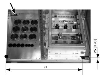
Side plates of the cabinet: 15 mm Back plate of the cabinet: 10 mm
