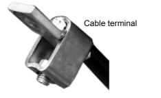
**WARNING!** If the wire size is less than  $95 \text{ mm}^2$  (3/0 AWG), a cable lug must be used. A cable of wire size less than  $95 \text{ mm}^2$  (3/0 AWG) connected to this terminal will loosen and may damage the drive.
