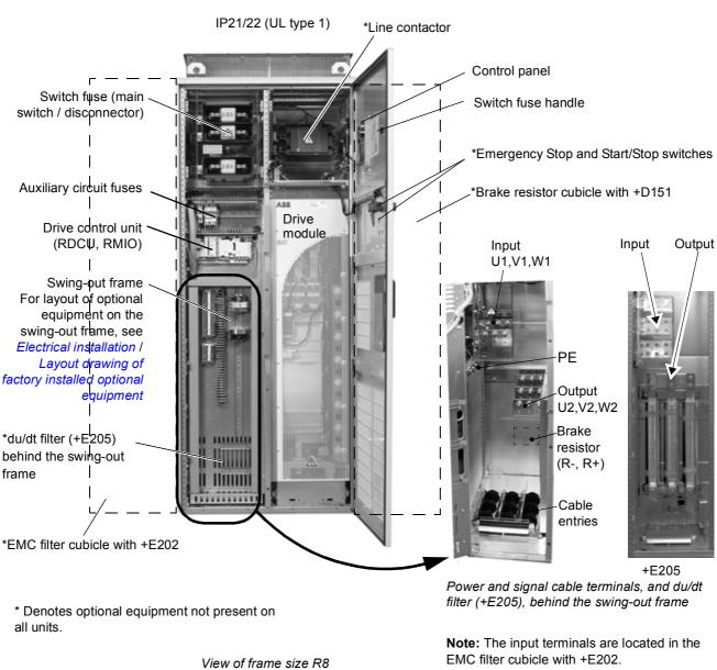
The ACS800-07/U7 is a cabinet-installed drive for controlling AC motors.
